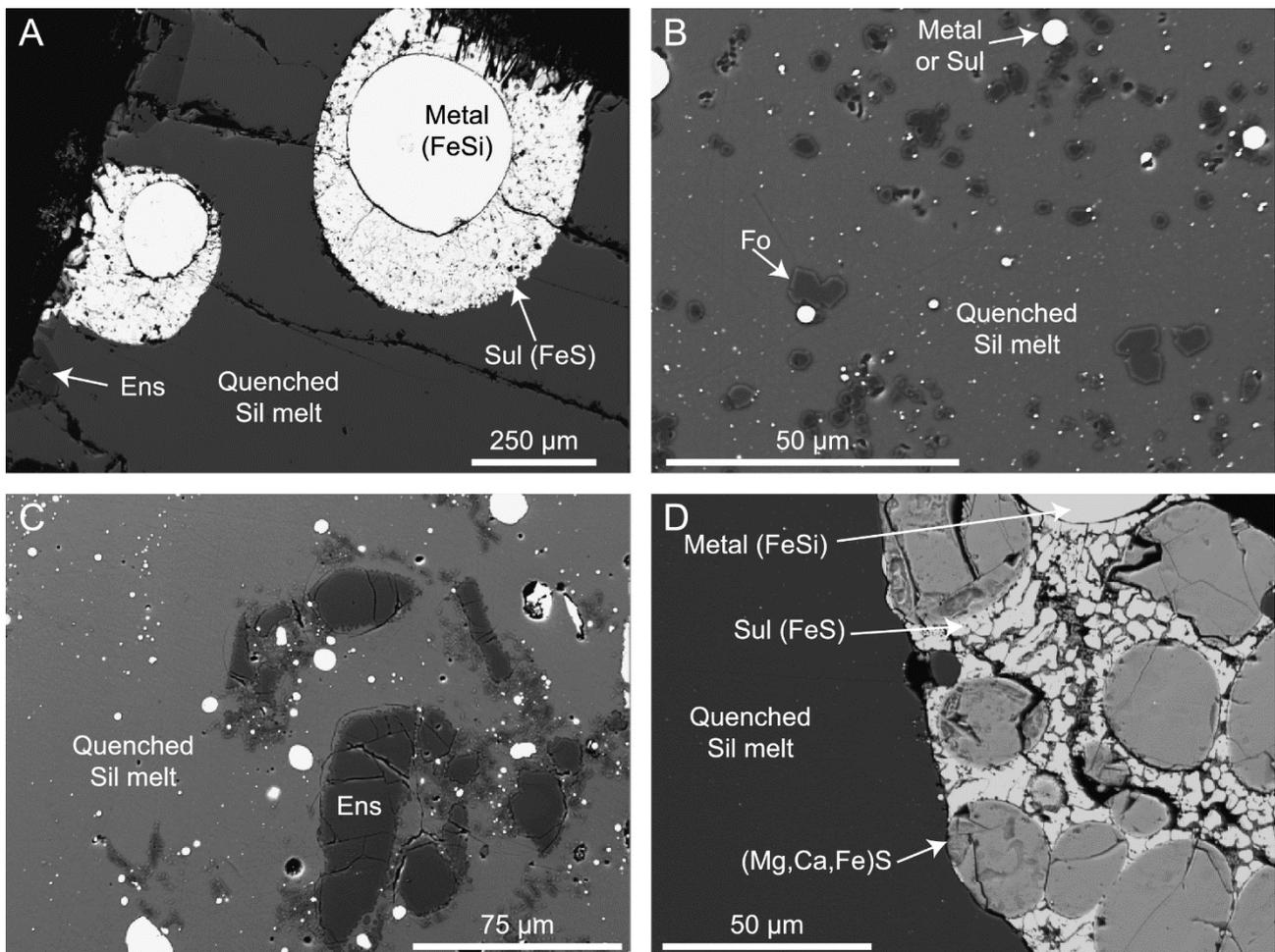
Back-scattered electron images of experimental products. A. Run A707; 1560 °C; 2 GPa. Sulfide melt is observed around droplets of metallic melt. Note the presence of quench crystals in the sulfide melts. Enstatite forms large crystals on the edges of the experimental charge. B. RY-14-1; 1250 °C; 0.3 GPa. Forsterite forms small crystals disseminated in
